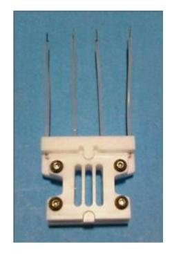
The advantage of the 4-electrode in-plane conductivity measurement is the ability to measure resistance due only to charge transport while excluding interfacial and charge transfer resistances. By considering only resistance due to ion transport, accurate assessment of in-plane membrane conductivity can be made.
