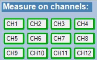
This panel in the main screen contains a toggle button for each channel determines which channels are participating in the measurement.
